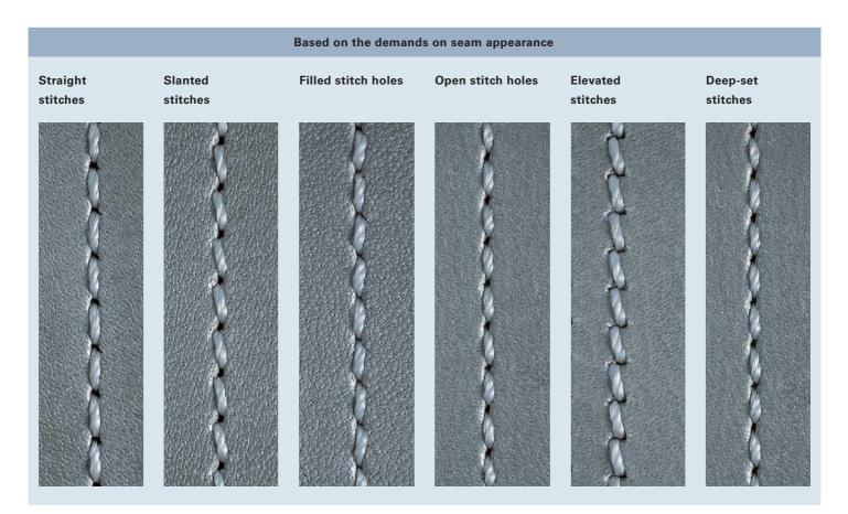
The pictures illustrating seams shown here and on the following pages, are based on the common threading direction from left to right. -○→ Seams were produced on leather of medium hardness.
