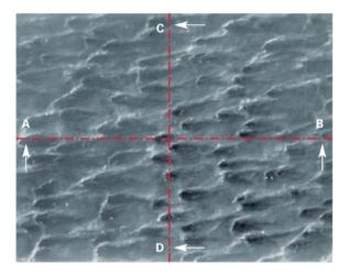
When using a needle with normal **cloth point (e.g. "R")** the stitch appearance will be different, and by what degree, depends on the sewing direction and properties of the leather.
